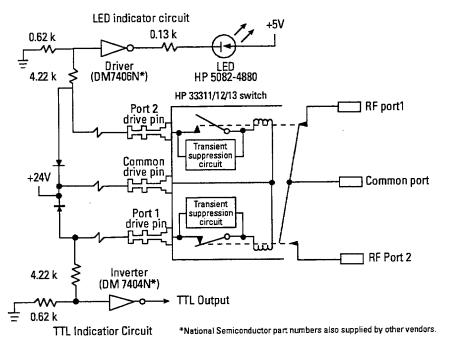
Figure 7. TTL and LED remote indicator circuits
